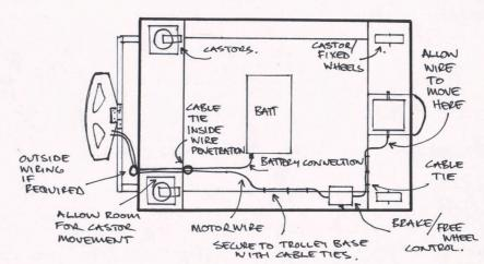
allow sufficient length of the motor lead cable to the motor to allow motor mount retraction as required. operate the motor bracket up and down a few times to check the wiring doesn't jam.
